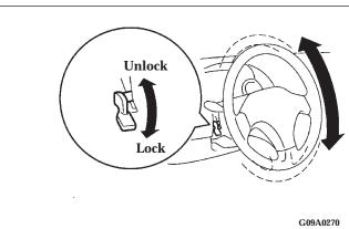
To adjust the steering wheel height, release the tilt lock lever while raising or lowering the steering wheel to the desired height.
